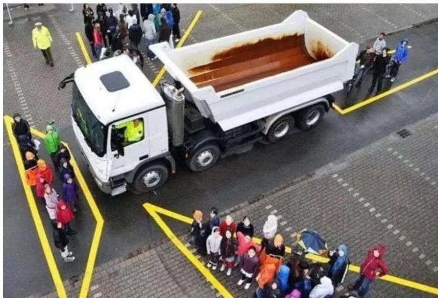
Figure 3:Blindspots of a truck
